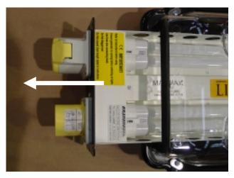
Separate the metal chassis from the plastic case assembly and withdraw the lighting cassette.
