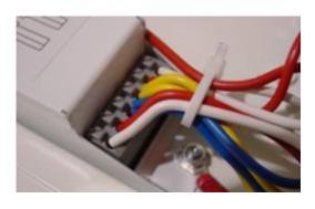
Replace the lamp holder wires in the correct sequence by depressing each retainer using a screwdriver and pushing each wire into place.
